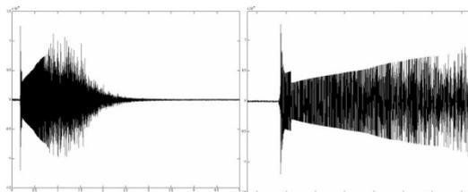
**Figure 2** – Automatic Gain Control modification on room impulse response profile
